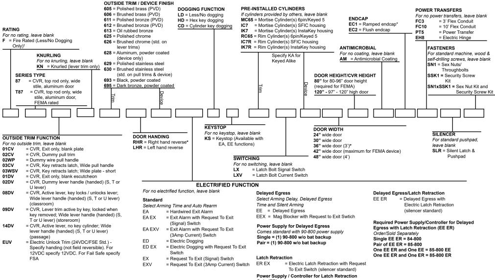
Fire-rated trims must be fail safe (FSA)
