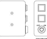
Attach to surface with flathead wood screws (included), using countersunk holes as template.
